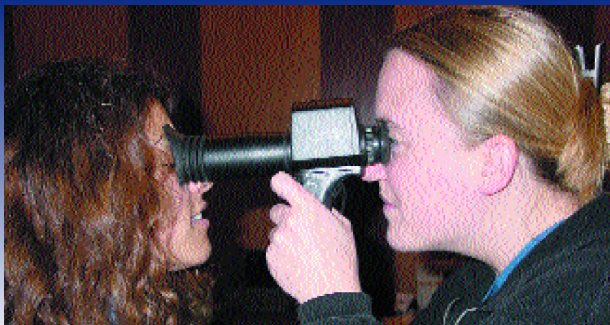
The Colvard Pupillometer measures the pupil size using infrared light.
